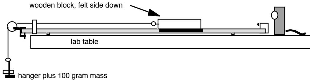
2. Make sure the track is level. A cart should not be rolling in either direction. Also, make sure that the string is attached to the pulley horizontally. (This can also be done on the lab table instead of the track.)
