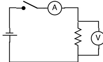
2. Vary the power until you are reading about .05 A in the resistor. Record the exact current and voltage. Remember to record the voltage and current as measured by the portable meters.
