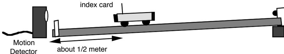
4. Open up LoggerPro. Start timing. After you hear the Motion Detector clicking, push the cart and let it go. Give the cart enough initial velocity so that it gets to within 10 cm of the raised end. Don't let the cart slam into the bottom of the ramp! (This may take a few trials.)
